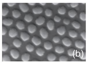
**Figure 1.** SEM image of the sample showing the Nb film containing the triangular array of V pillars. (a)  $\times 50~000$  and (b)  $\times 40~0000$ . The sample was rotated  $30^{\circ}$  from the beam direction to observe the V pillars.
