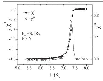
**Figure 2.** Screening  $\chi'(T)$  (full symbols, left axis) and losses,  $\chi''(T)$  (open symbols, right axis) at zero dc field for  $h_{\rm ac}=0.1$  Oe and f=1 kHz.
