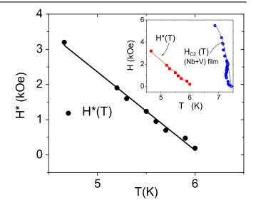
**Figure 5.**  $H^*$  versus T (black full circles; the line is a guide to the eye). The inset shows  $H^*(T)$  and the sample  $H_{C2}(T)$  in red full squares and blue full circles, respectively.
